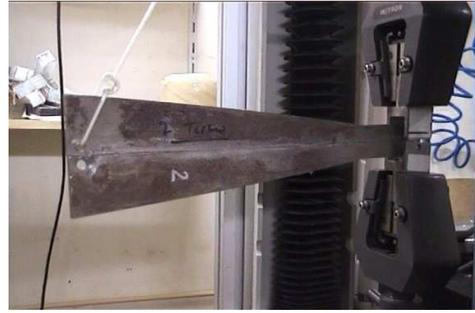
Fig.5. Experimental TDCB specimen
