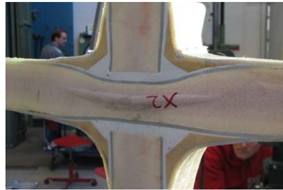
Fig. 12. Large deformations in the core and failure of upper overlaminations in the X2 1 specimen.
