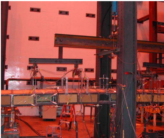
Fig. 2. Experimental setup for testing the hybrid ship hull model
