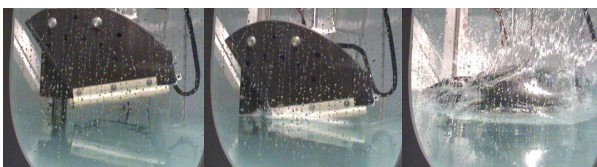
Fig. 6. Typical slamming event in SSTS
