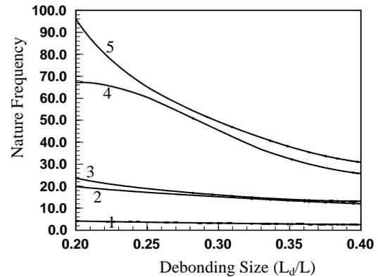
Fig.2 Effect of debonding size on natural frequency
