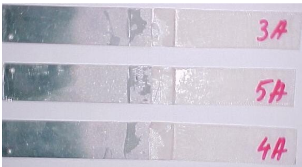
Fig. 20. Hybrid (aluminium/wet molded laminates, 4 layers) single lap joint aspect after static testing for L_a = 12.5 \text{ mm}
