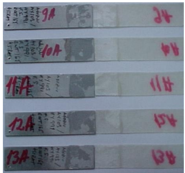
Fig. 19. Hybrid (aluminum/wet molded laminates, 4 layers) single lap joint aspect after static testing, for L_a = 25 \text{ mm}
