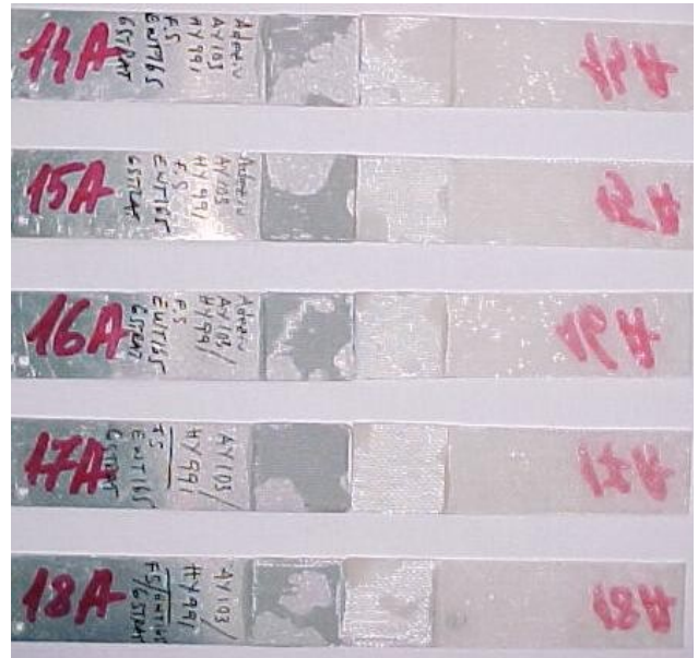
Fig. 18. Hybrid (aluminum/wet molded laminates, 6 layers) single lap joint aspect after static testing, for L_a = 25 \text{ mm}
