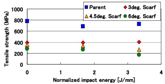
Fig.10 Residual tensile strength of scarf joints
