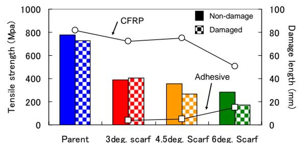
Fig. 17 Relationship between residual strength and crack length.
