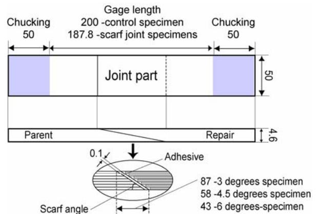
Fig.3 Schematic of scarf joint specimen for tensile test.
