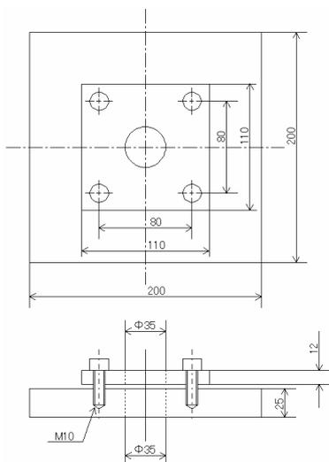
Fig.7 Impact support base for tensile specimen
