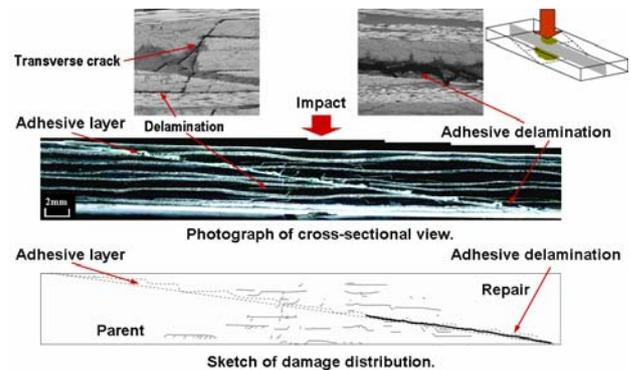
Fig. 16 Cross-sectional observation of 6-degrees specimen.
