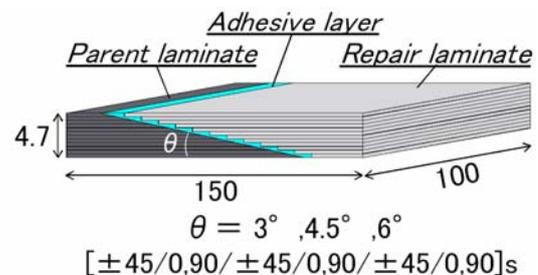
Fig.4 Schematic of scarf joint specimen for compressive test.
