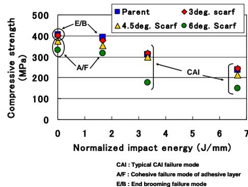
Fig.12 Residual compressive strength of scarf joints
