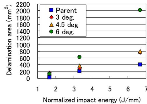
Fig.18 Relation between normalized impact energy and delamination area of compressive specimen
