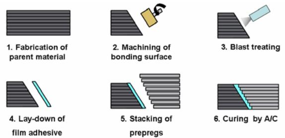
Fig.2 Fabrication process of scarf joint
