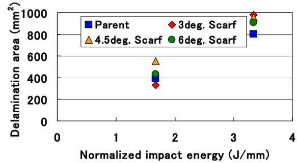
Fig.14 Relation between normalized impact energy and delamination area of tensile specimen
