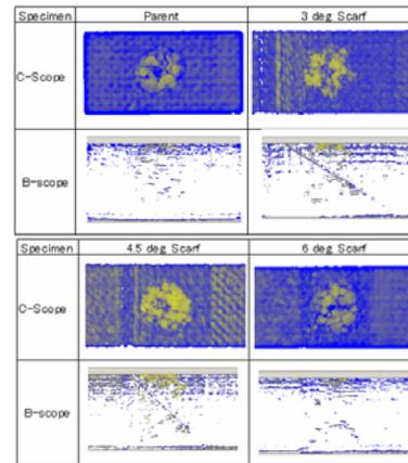
Fig.15 C and B scope images by ultrasonic testing of tensile specimen (applied impact energy of 3.34J/mm)
