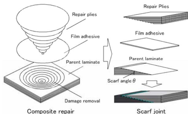
Fig.1 Simplification of composite repair part.
