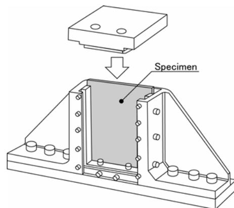
Fig.5 Compression test fixture
