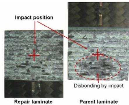
Fig.11 Failure mode of 6deg. scarf specimen after tension test (applied impact energy of 3.34J/mm)
