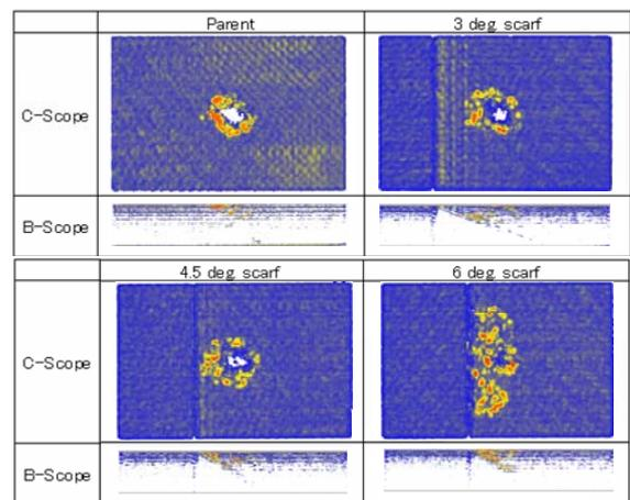
Fig.19 C and B scope images by ultrasonic testing of compressive specimen (applied impact energy of 6.67J/mm)
