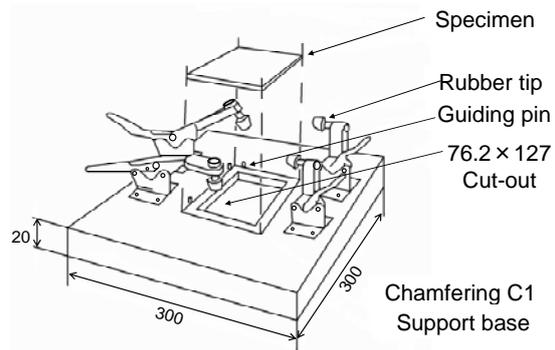
Fig.8 Impact support base for compressive specimen
