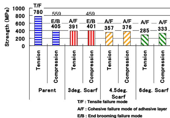
Fig.9 Results of tensile and compressive specimens
