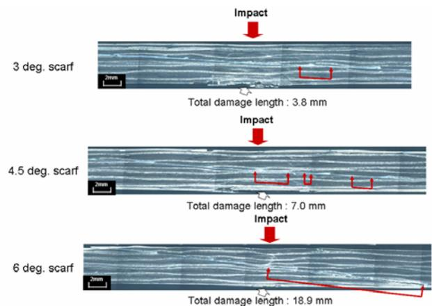
Fig. 16 Cross-sectional observation of scarf joint
