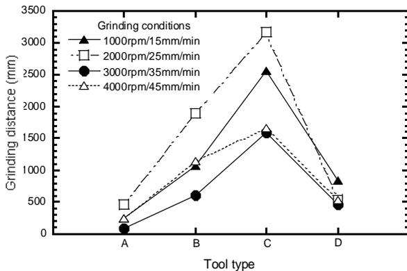
Fig.6. The available grinding distance with four different grinding conditions for four diamond composite tools.
