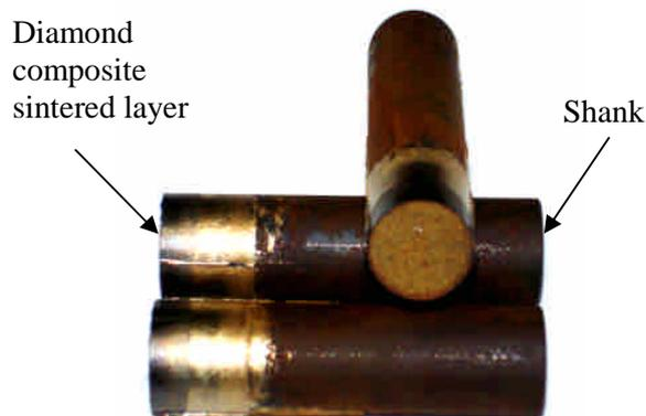
Fig.1. The bronze-bonded diamond composite tools
