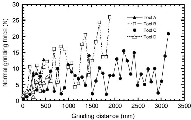
Fig.4. The variations of the normal grinding forces with the available grinding distance between two dressings during dry grinding BK7 glass at the spindle speed of 2,000 rpm and the table speed of 25 mm/min.
