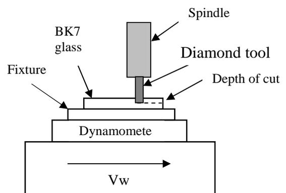
Fig.3 Geometry of the grinding kinematics for the bronze-bonded diamond composite tools.
