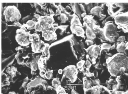
Fig.2. The microstructure on the fracture surface for diamond composite tool C.
