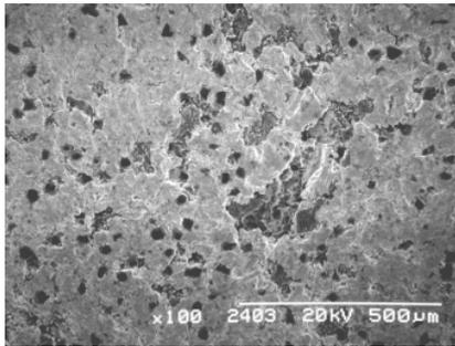
Fig.8. The worn flat appearance with many flat diamonds on the matrix produced for tool A at the spindle speed of 4000 rpm and the table speed of 45mm/min.
