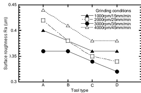
Fig.10. The average surface roughness of the workpiece before the near end of dry grinding for four diamond tools at four different grinding conditions.
