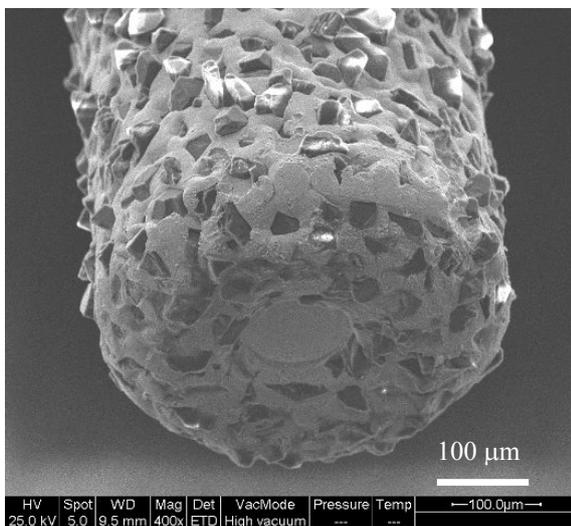
(a) For the topcoat layer composed of Ni coating
