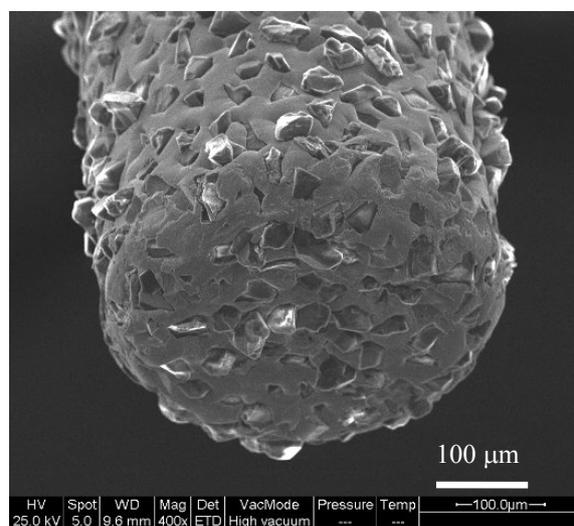
(b) For the topcoat layer composed of Ni-based CNT composite coating
