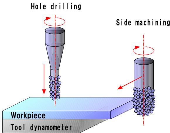
Fig. 2 Schematic illustration of side machining and hole drilling for testing tool life.
