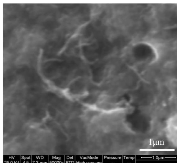
Fig. 4. SEM image of CNT composite coating surface etched by acid.
