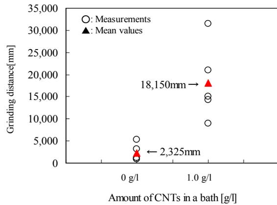
Fig. 7. The tool life of electroplated diamond tool versus amounts of CNTs in bath.
