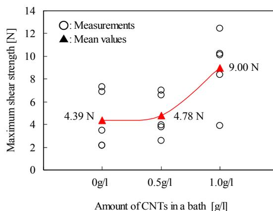
Fig. 6. Grain retentivity of coatings versus amounts of CNTs in bath.
