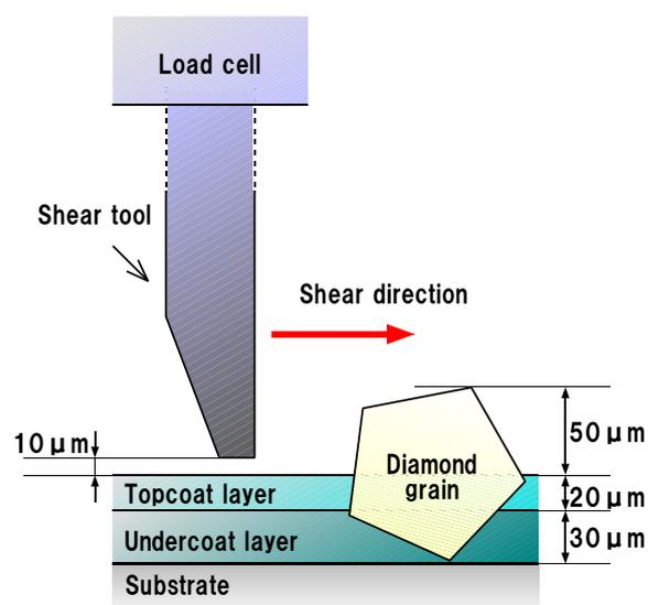
Fig. 1 Schematic illustration of shear test for grain retentivity evaluation using a bondtester.
