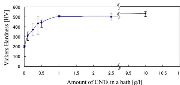
Fig. 5. Vickers hardness of coatings versus amount of CNTs in bath.
