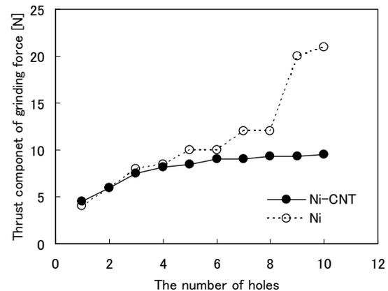
Fig. 10 Transition of the maximum grinding force (thrust component) for  $\phi 0.5$  mm hole drilling.
