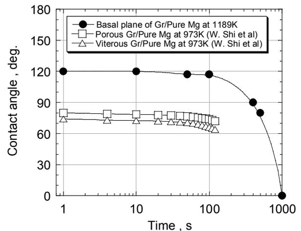
Fig. 7 Change in the contact angle between the basal plane of graphite and molten magnesium
