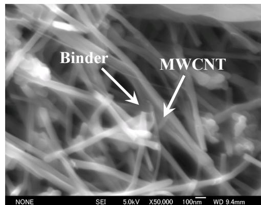
Fig. 13 Microstructure of the MWCNT preform (Vf: 25%, Binder addition: 50wt.%)
