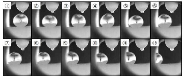
Fig. 9 Change in the shape of the droplet of molten magnesium on the MWCNT preform
