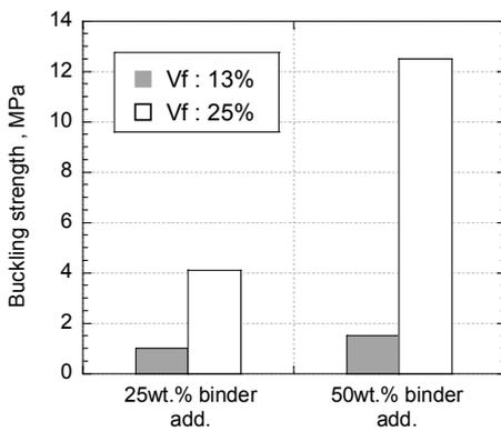
Fig. 11 Relationship between the buckling strength of the MWCNT preform and quantity of the binder addition
