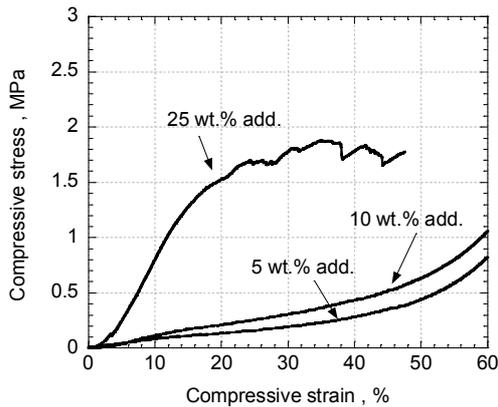
Fig. 10 Compressive stress - strain curve of the obtained MWCNT preform
