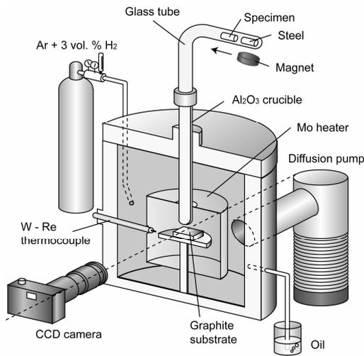
Fig. 3 Schematic illustration of the sessile drop device
