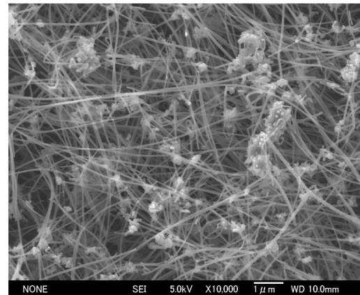
Fig. 2 Microstructure of MWCNT
