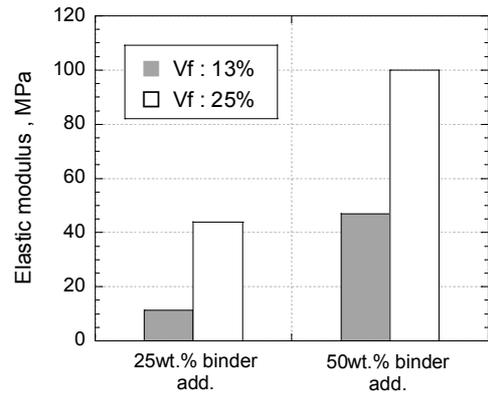
Fig. 12 Relationship between the elastic modulus of the MWCNT preform and quantity of the binder addition
