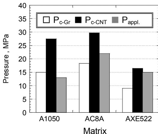
Fig. 11 Relationship between the estimated threshold pressure and the applied pressure to the MWCNT preform
