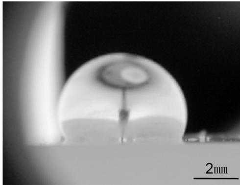
Fig. 4 Shape of the molten aluminum droplet on the basal plane of graphite
