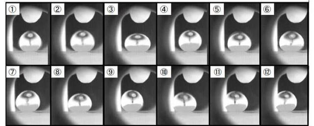
Fig. 8 Change in the shape of the droplet of molten aluminum on the MWCNT preform
