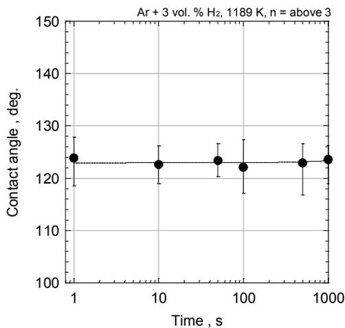
Fig. 5 Change in the contact angle between the basal plane of graphite and molten aluminum
