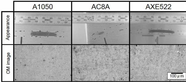
Fig. 14 Appearance of cross section of the MWCNT reinforced aluminum, magnesium alloy composites
