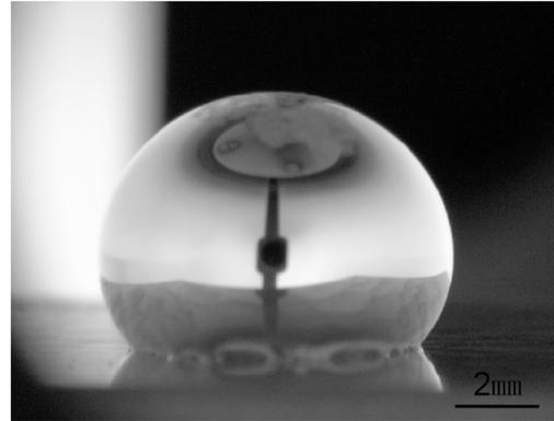
Fig. 6 Shape of the molten magnesium droplet on the basal plane of graphite
