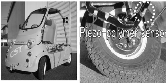
Fig. 2. The experimental vehicle and the sensor
