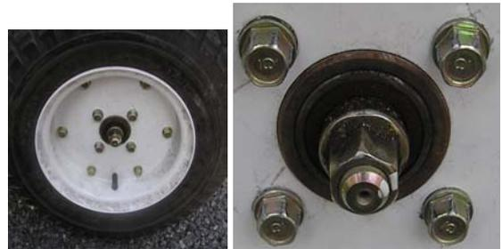
Fig. 9. The bolts joint a tire-wheel to a hub
