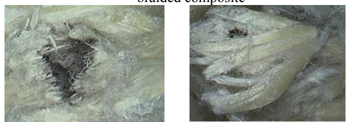
Damage morphology near penetration hole in striking side Damage morphology near penetration hole in distal side (2) Local magnification of damage pattern around the perforating hole
