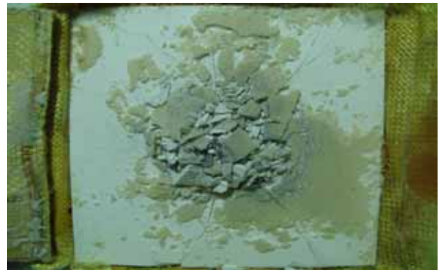
Fig.7 4mm thickness ceramic (Alumina 15%)
