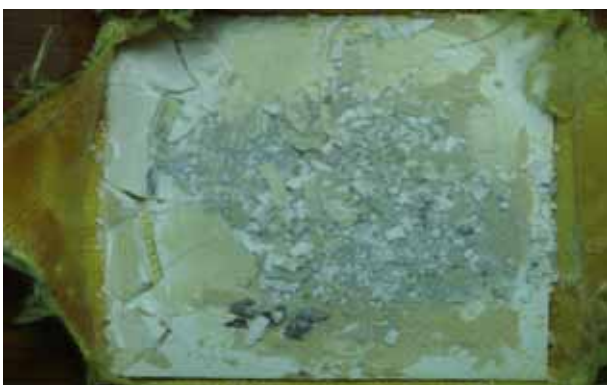
Fig.6 4mm thickness ceramic plane (5% z_r, o_2 )
