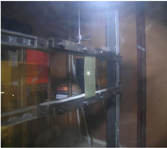
Fig. 1 Ballistic Impact Test on Composite Plate
