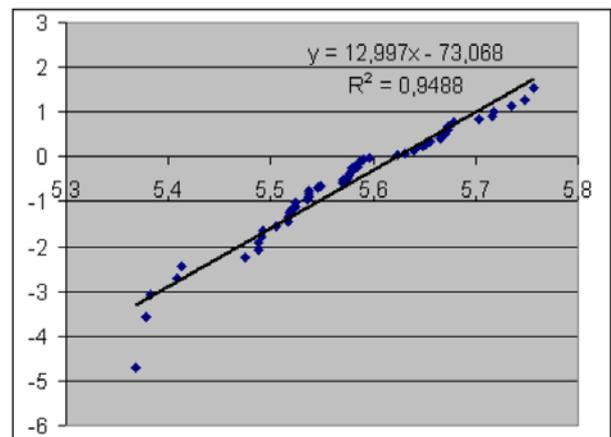
Fig. 13. Experimental curve for Weibull modulus
