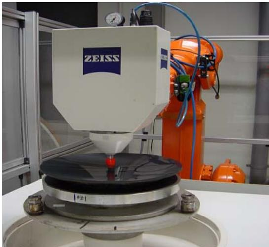
Fig. 14. Mirror during polishing
