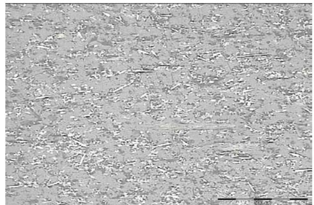
Fig. 1. REM microphotograph of the greenbody
