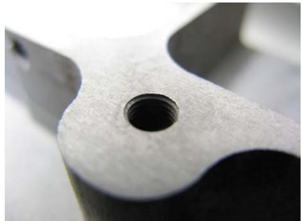
Fig. 17. HB-Cesic® thread inside structure
