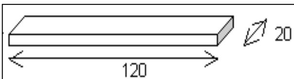
Fig. 12. Size of HB-Cesic® 4-point bending samples
