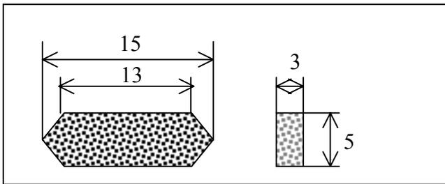
Fig. 7. Shape of the CTE samples
