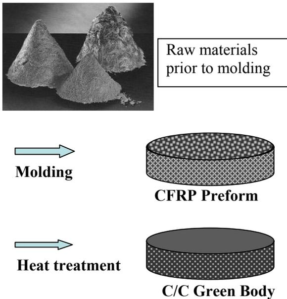
Fig. 4. Manufacturing process of the new C/C raw material
