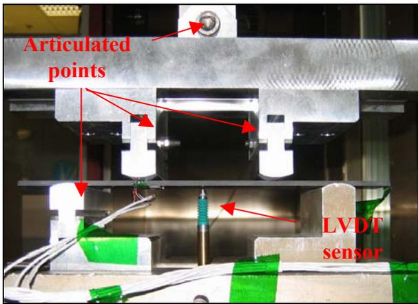
Fig. 11. Sample in 4-point bending test configuration at TAS. Test-setup shown is for a sample of length 240 mm. The HB-Cesic® tests were made with samples of length 120 mm
