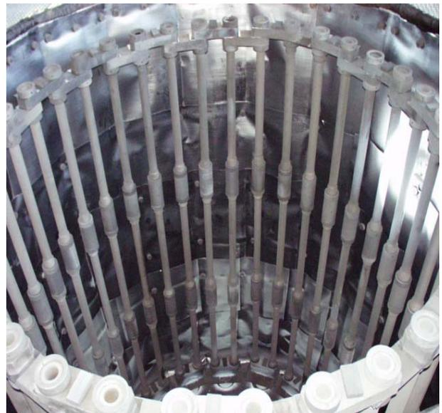
Fig. 3. Heater unit designed for best thermal homogeneity
