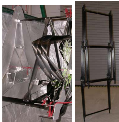
Fig. 2. Partially deployed concentrated strain structures.
