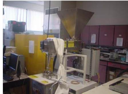
Fig.11. Microtech UTM100 cryo-grinder
