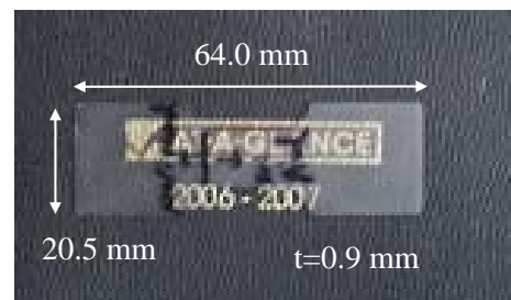
Fig.13. Pure dog-bone shape PMMA specimen
