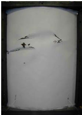
Fig. 15. Failed curved panel
