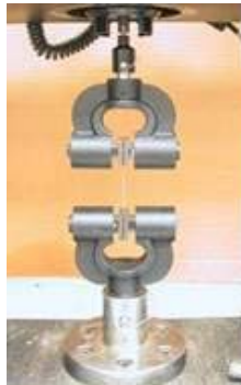
Fig. 7. Tensile testing setup for Nylon-66
