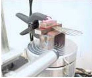
Fig. 8. Flexural test setup for phenomenological wings
