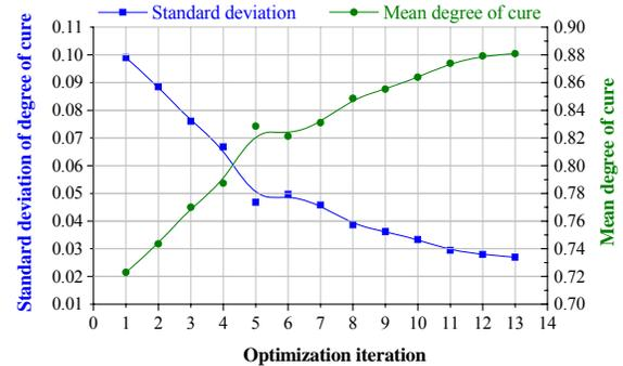
Fig. 16. Mean degree of cure and standard deviation of degree of cure for C section at die exit.
