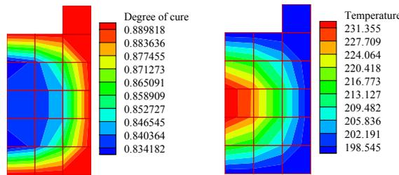
Fig. 12. Degree of cure and temperature profiles at pull speed 5mm/sec.
