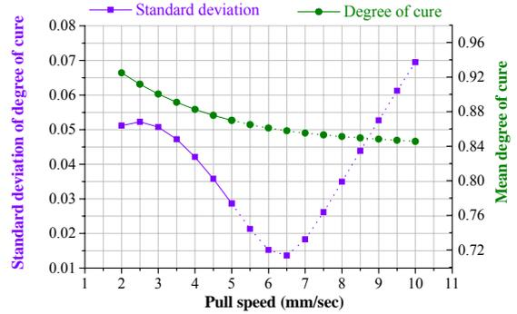
Fig. 10. Mean and standard deviation of degree of cure for C-section at die exit as a function of pull speed.
