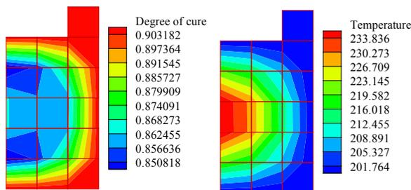
Fig. 21. Contours in C-section at the die exit after optimization at 1000 Watts heater power.
