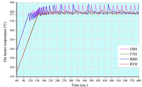
Fig. 15. Fluctuations in die heater temperature due to ‘switch-on & off’ power control.
