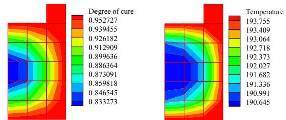
Fig. 11. Degree of cure and temperature profiles at pull speed 2mm/sec.
