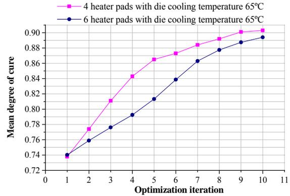
Fig. 7. Comparison of mean degree of cure for C section at the die exit based on heater arrangement.
