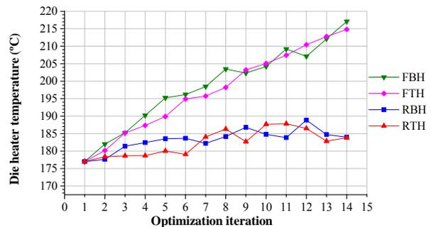
Fig. 17. Die heater temperatures for every optimization iteration.
