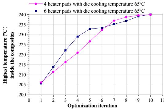
Fig. 9. Highest temperature in C-composites for two different heater arrangements.
