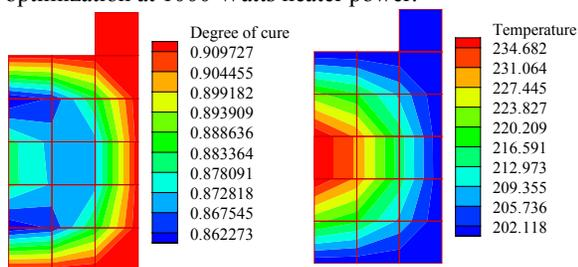
Fig. 22. Contours in C-section at the die exit after optimization at 2000 Watts heater power.
