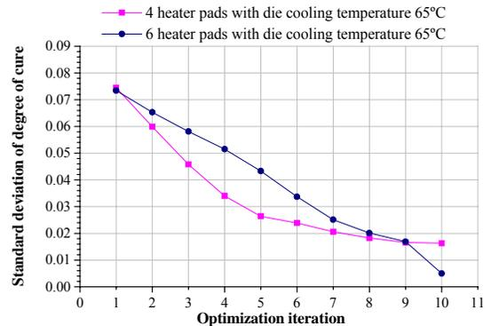
Fig. 8. Comparison of Standard deviation of mean degree of cure for C section at the die exit based on heater arrangement.
