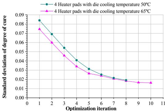
Fig. 5. Standard deviation of degree of cure for C section for two different die cooling temperatures.
