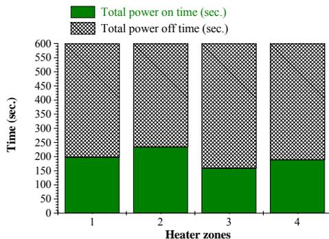
Fig. 14. Heater zones and total power-on and -off time seconds at the end of 1<sup>st</sup> optimization iteration.
