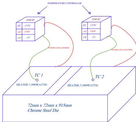
Fig. 13. Schematic showing concept of controlling die-heater temperature through power supply to die heaters.
