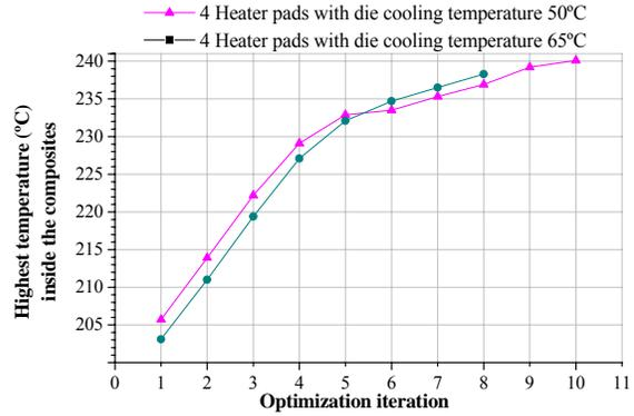
Fig. 6. Highest temperature in C-composites as a function of optimization iterations.
