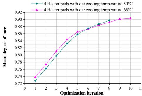
Fig. 4. Mean degree of cure for C section at die exit for two different die cooling temperatures.
