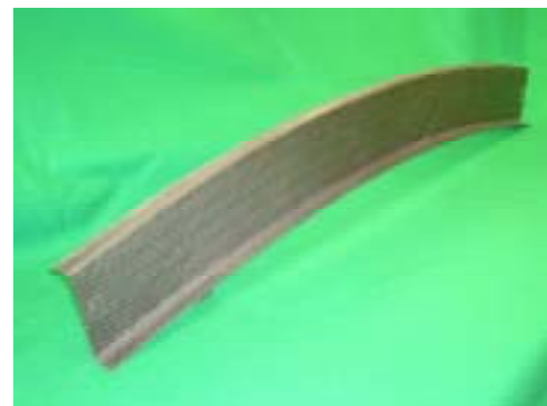
Fig. 3. Z-section composite frame member fabricated by UV-cured RTM process
