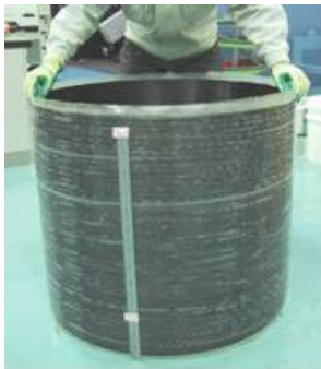
Fig.5. Trial composite parts fabricated by FW/UV-curing process
