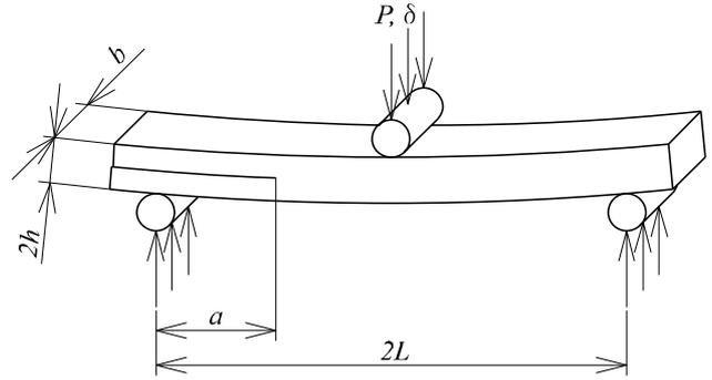
Fig. 3. Schematic of ENF specimen
