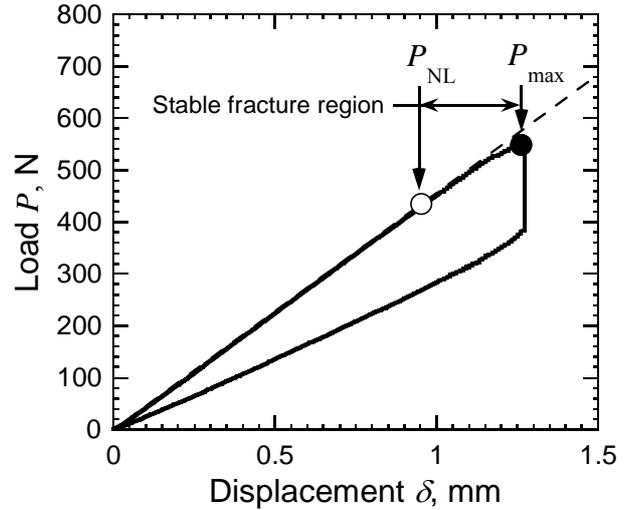
Fig. 4. Typical load-displacement relation at the first loading step (material; Z1).
