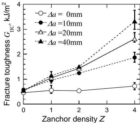
Fig. 7. Effect of Zanchor density on the mode II fracture toughness
