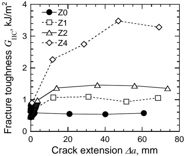
Fig. 6. Crack resistance curves (R-curve) of Zanchor reinforced composites.
