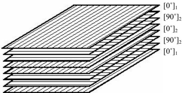
Fig. 2. Stacking sequence of the composite
