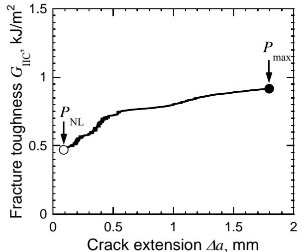
Fig. 5. Crack resistance curve (R-curve) of Zanchor reinforced composite during the initial stage of crack extension (material; Z1).
