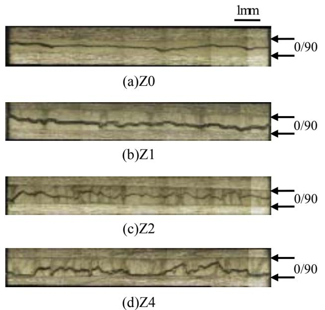
Fig. 8. Effect of Zanchor density on microscopic fracture morphology (distance from the end of crack;  $\xi = 10$  mm, crack growth direction;  $\otimes$ ).
