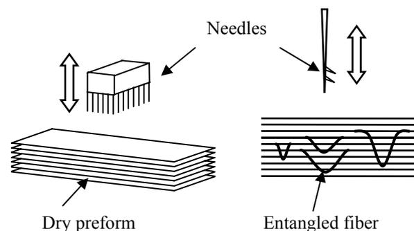
Fig. 1. Schematic of Zanchor technology
