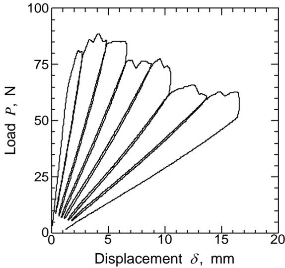
Fig. 3. Load-displacement responses of the Zanchor reinforced composite, Z1, in DCB tests.
