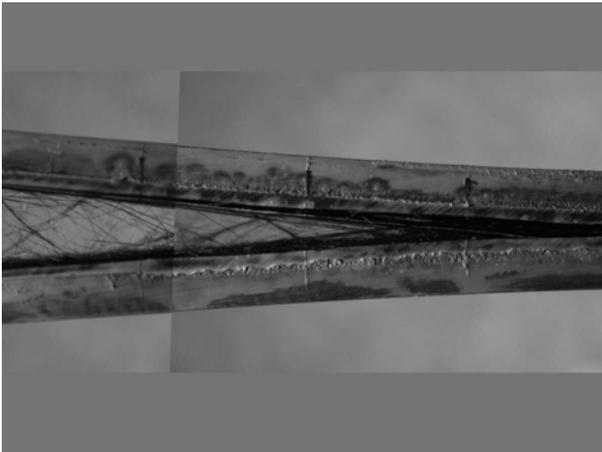
Fig. 8. Macroscopic fracture morphology of the Zanchor reinforced composites, Z1, under mode I loading (crack growth direction  $\Rightarrow$ ).
