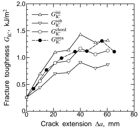
Fig. 5. Comparison of fracture toughness of the Zanchor reinforced composite, Z1, in DCB tests.
