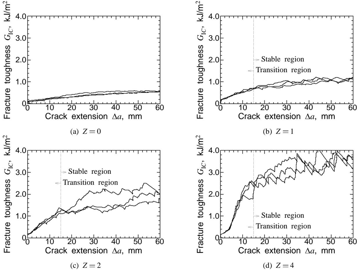
Fig. 6. Crack resistance curve of the composites under mode I loading.
