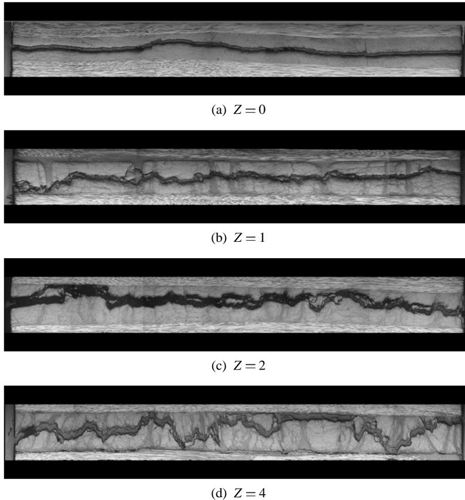
Fig. 10. Effect of Zanchor density on mode I fracture morphology of the Zanchor reinforced composites (cutting position  $\xi = 10$  mm, crack growth direction  $\otimes$ ).
