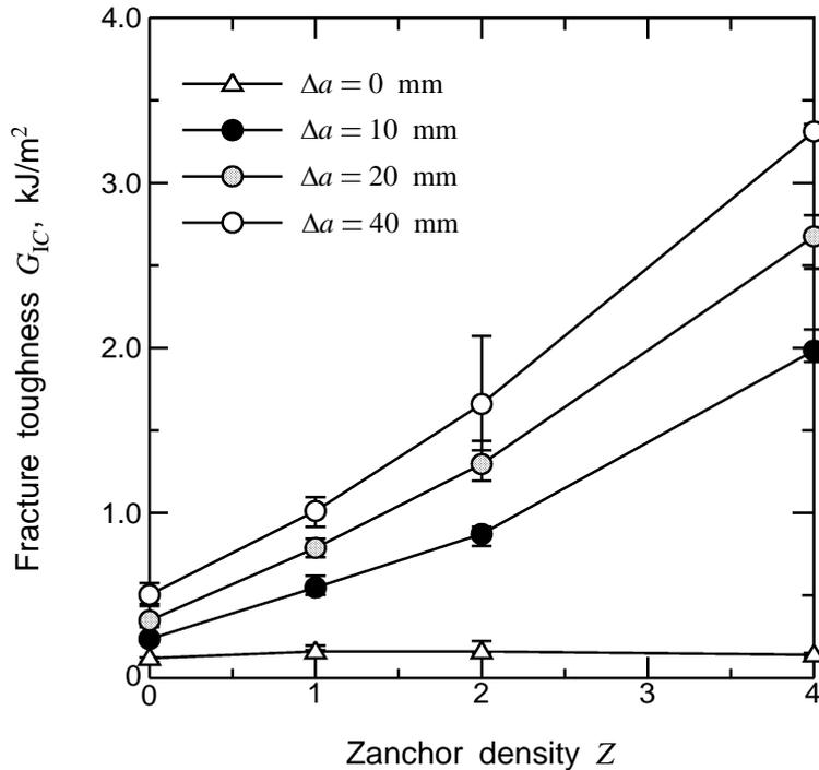
Fig. 7. Effect of Zanchor density on mode I fracture toughness of the Zanchor reinforced composites.
