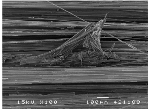
Fig. 9. Microscopic fracture morphology of the Zanchor reinforced composites, Z2, under mode I loading (crack growth direction  $\Rightarrow$ ).
