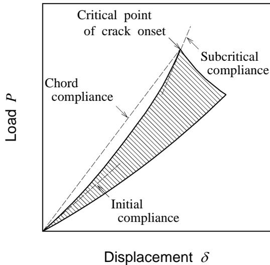
Fig. 4. Definition of loading point compliance in DCB tests.
