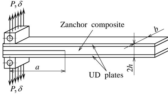
Fig. 2. Schematic drawing of DCB specimen.
