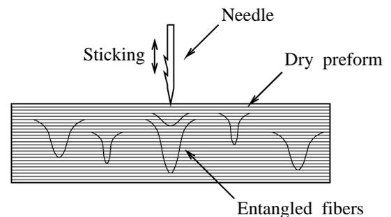
Fig. 1. Schematic drawing of Zanchor process.
