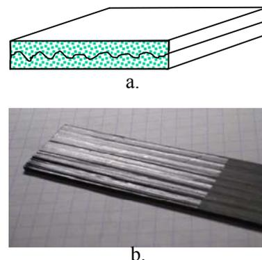
Fig. 2 a) schematic of nesting b) evidence of nesting on the fracture surface of an interlaminar toughness specimen
