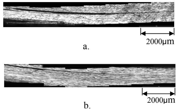
Fig. 17. Micrographs of the edge of the miniature 4ENF specimen: a) film insert specimen b) natural starter crack specimen
