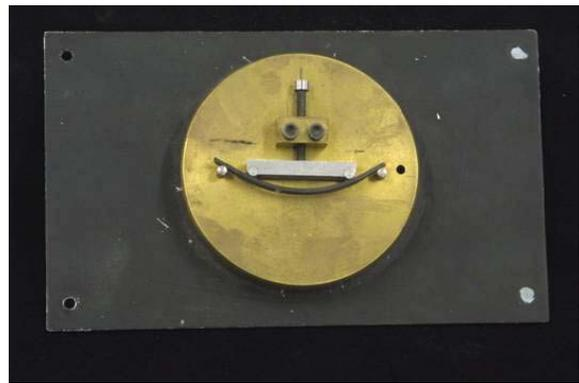
Fig. 16. Microscope stage and miniature 4ENF test
