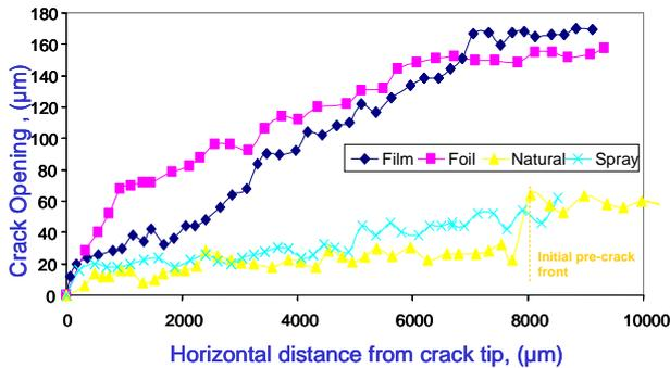
Fig. 18. Crack opening profile measured in miniature 4ENF specimens
