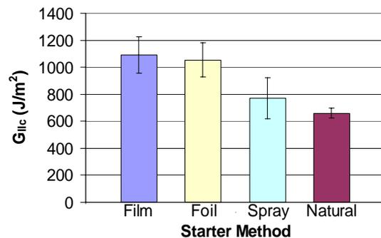
Fig. 11. Initiation values of  $G_{IIc}$  for various starter crack methods
