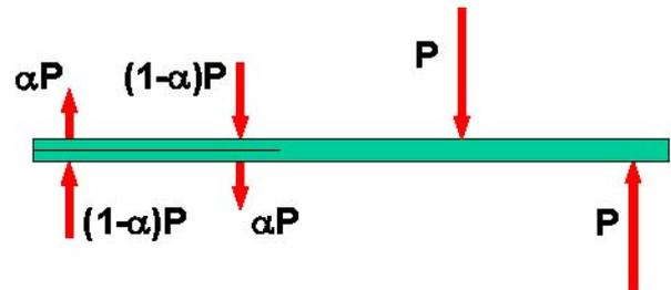
Fig. 3. Modified 4-ENF loading configuration
