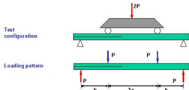
Fig. 1 Conventional 4ENF test (for the tests reported here  $b=30\text{mm}$ ,  $c=60\text{mm}$ )
