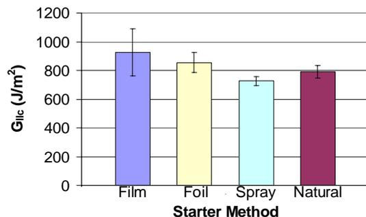
Fig. 12. Propagation values of  $G_{IIc}$  for various starter crack methods
