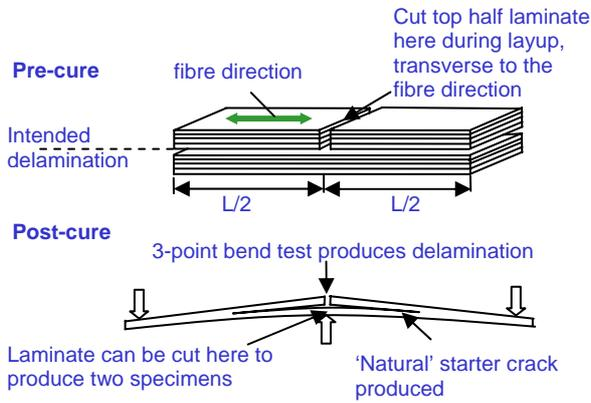
Fig. 5. Method for producing natural starter crack
