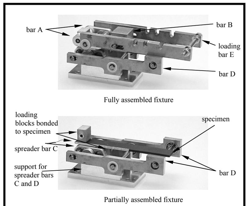
Fig. 4. Loading strategy and test fixture for modified 4ENF
