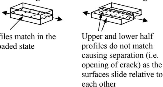
Fig. 15. Effect of nesting on separation of sliding surfaces
