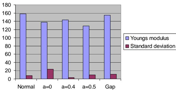
Fig. 8. Flexural Young's modulus from conventional and modified 4-ENF tests
