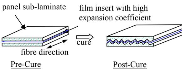
Fig. 14. Schematic showing possible mechanism of nesting production in film insert specimens
