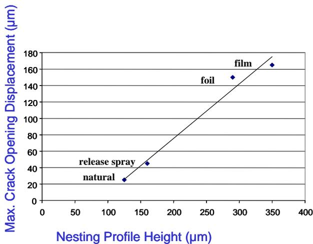
Fig. 19. Maximum crack opening displacement versus height of nesting profile
