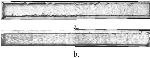
Fig. 13. Transverse micro-sections showing surface profile for a) film insert and b) natural starter crack
