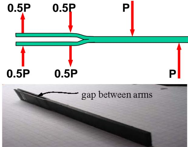
Fig. 6. ‘Gap’ specimen used in modified 4-ENF specimen
