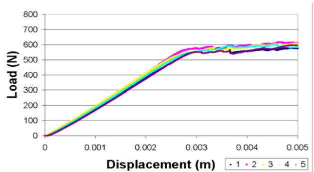
Fig. 10. Load-displacement plots for natural starter crack specimens
