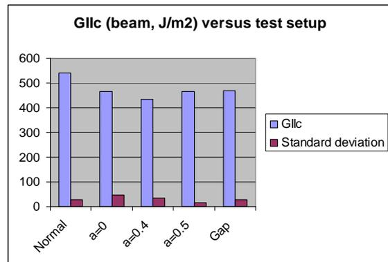
Fig. 7. Measured  $G_{IIC}$  for conventional and modified 4-ENF tests
