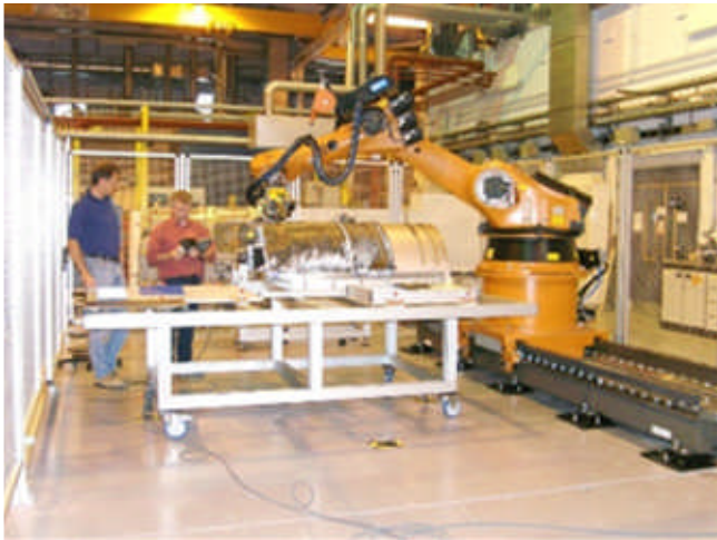
Fig. 3. QinetiQ stitching robot on 3m rail
