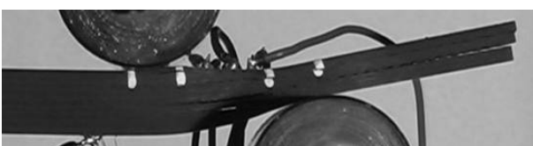
Fig. 18 – Failure in the three point bending test
