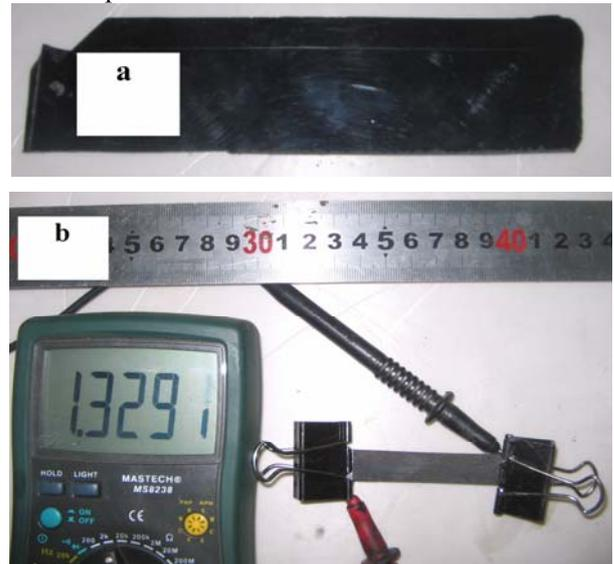
Fig. 4. 8.0×2.0×0.2 (cm<sup>3</sup>) 8wt.% MWNTs composite (a), and its surface resistivity is 80 $\Omega$ ·cm (b)
