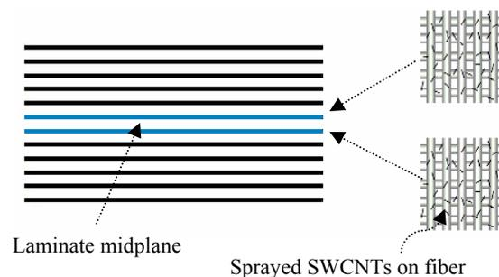
Fig. 1. Nanocomposite laminate cross-section
