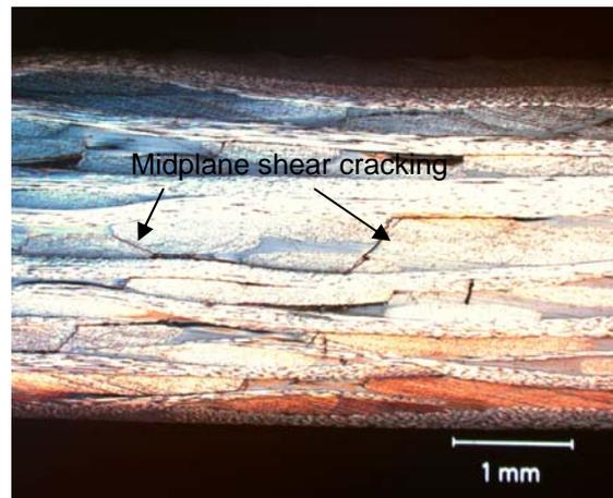
Fig. 4. Carbon fiber without SWCNTs
