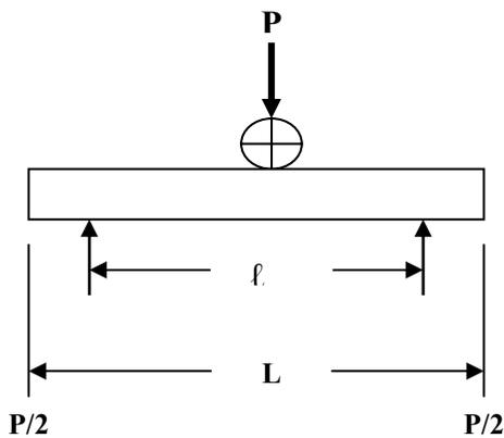
Fig. 2. Short beam shear test loading configuration
