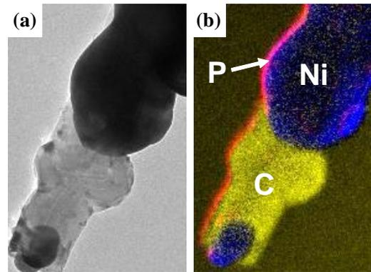
Fig. 3. (a) TEM BF image and (b) EELS map of Ni-P/CNFs with uncoated layers
