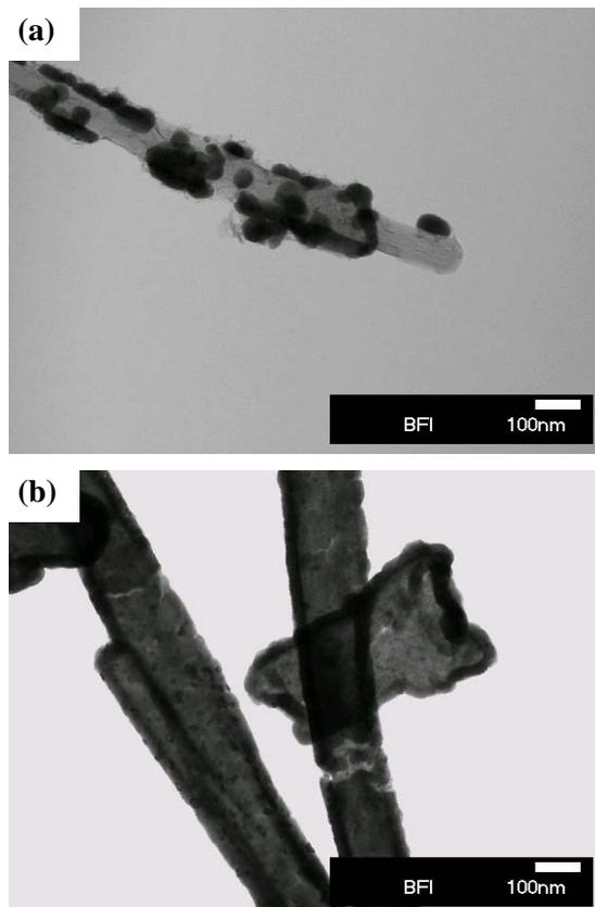
Fig. 2. TEM BF images of Ni-P/CNFs (a) during process (b) after process
