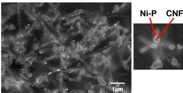
Fig. 8. Cross section of Ni30 composites
