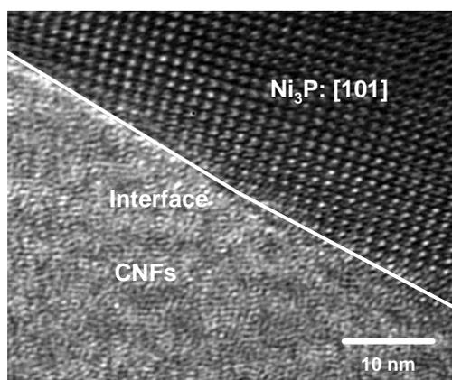
Fig. 5 HR TEM image containing the interface region of Ni-P coated CNFs.
