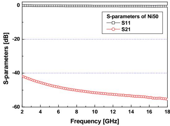
Fig. 10. S-parameters of Ni50
