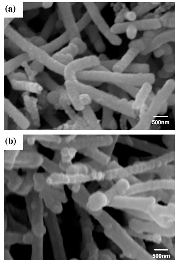
Fig. 4. SEM images of (a) as-fabricated Ni-P/CNFs (b) heat-treated Ni-P/CNFs
