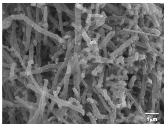
Fig. 6. SEM image of Ni-Fe/CNFs
