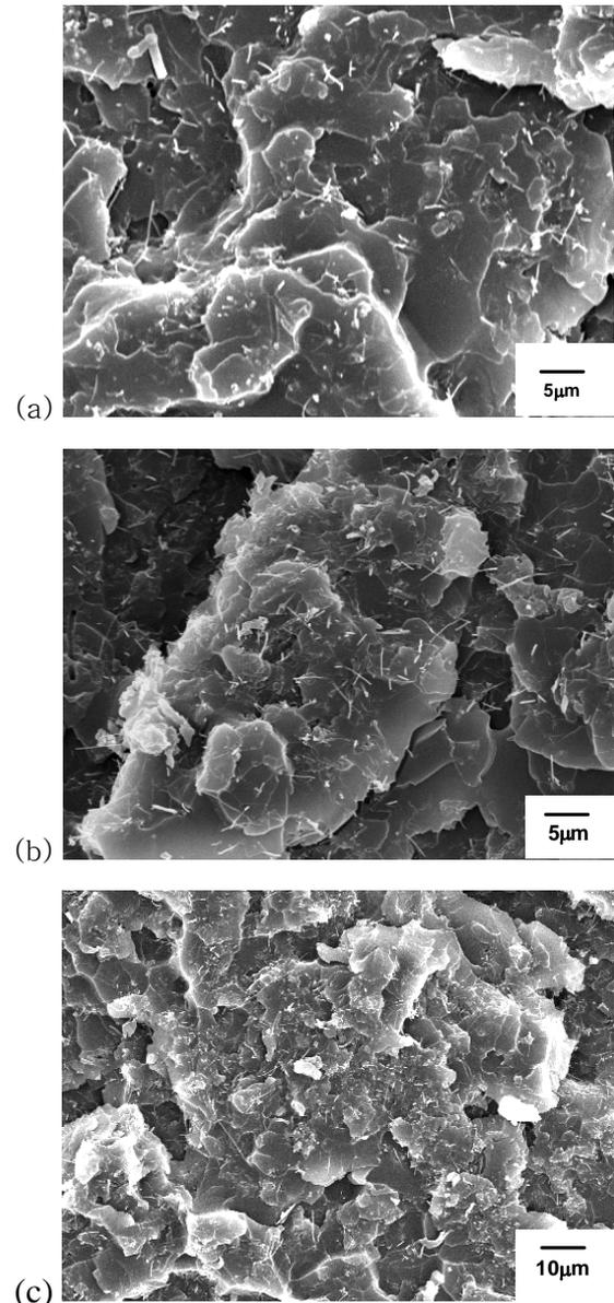
Fig. 3. SEM micrographs revealing fracture surfaces with 2.0 wt% VGCF contents. (a) with homogenizer method, raw VGCF, (b) with ultrasonic method, raw VGCF, (c) with sonic method, plasma treated VGCF.
