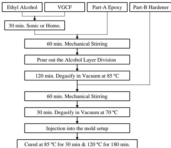
Fig. 2. The manufacturing process of VGCF/epoxy composite plates.
