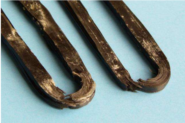
Fig. 10. Two loop samples after test with washers
