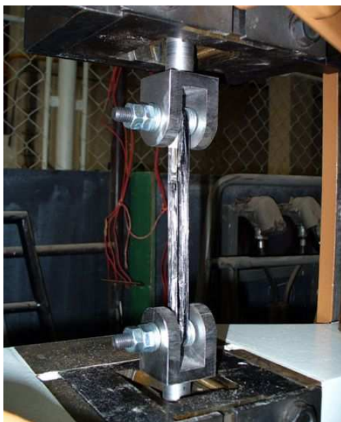
Fig. 6. Loop sample gripped in testing machine
