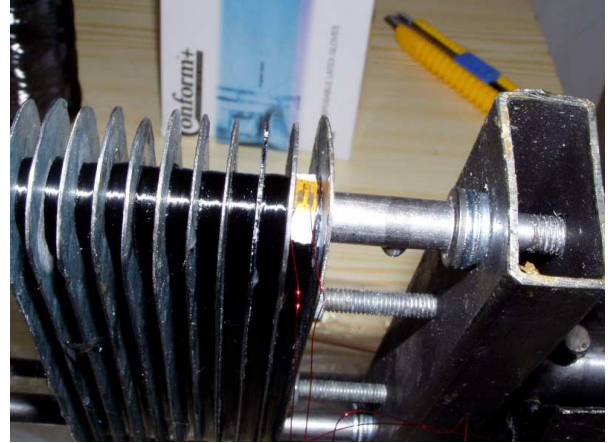
Fig. 12. Manufacturing process of loops and placement of strain gauge
