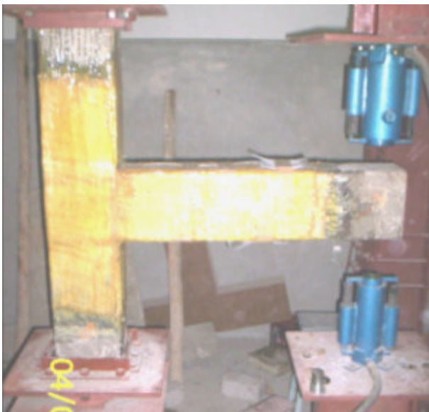
Fig. 4. Setup to apply cyclic action
