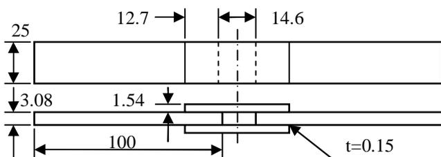
Fig. 1: Short term stress relaxation specimen. All dimensions are in mm.
