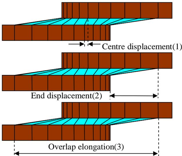
Fig. 9: Creep measurement of overlap.
