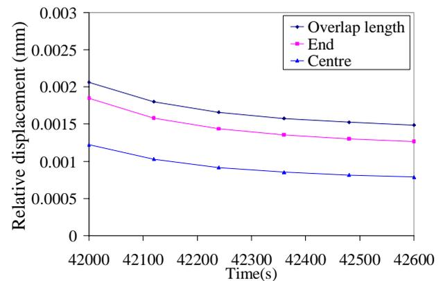
Fig. 11: 20-ply creep results at unload after ten load cycles
