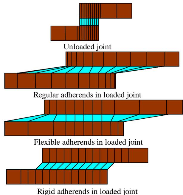
Fig. 6: Effect of adherend stiffness on adhesive strain
