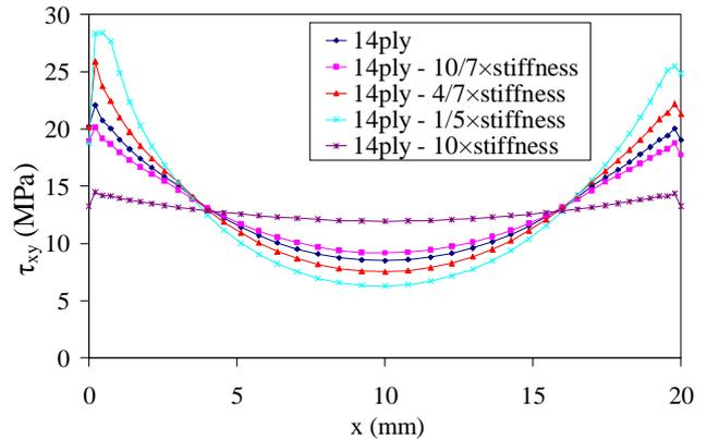
Fig. 5: Effect of material stiffness on shear stress
