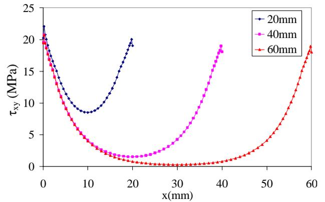
Fig. 8: Effect of joint length on initial shear stress
