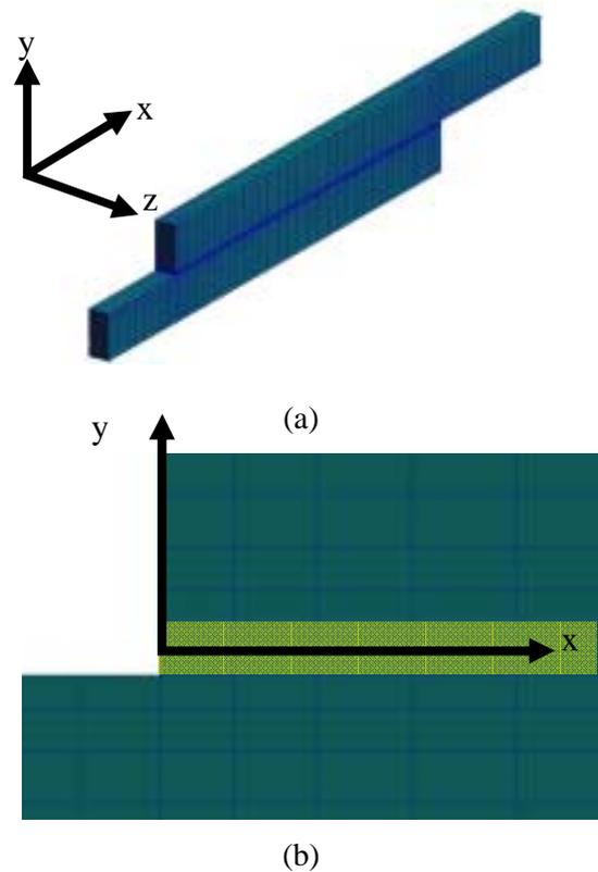
Fig. 3: Finite element model; (a) Whole model; (b) Overlap end with origin.
