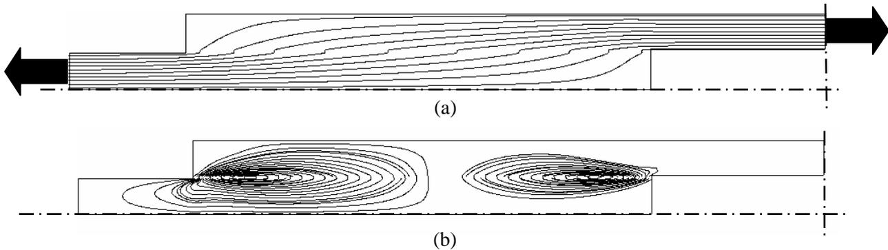
Fig. 17: Load path in quarter of joint; (a) Loaded; (b) Unloaded.
