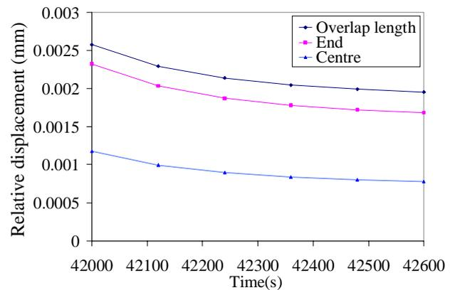
Fig. 10: 14-ply creep results at unload after ten load cycles
