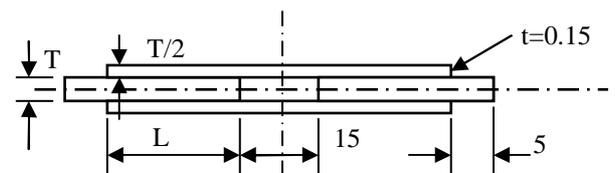
Fig. 4: Joint geometry used in FEM. All dimensions are in mm.
