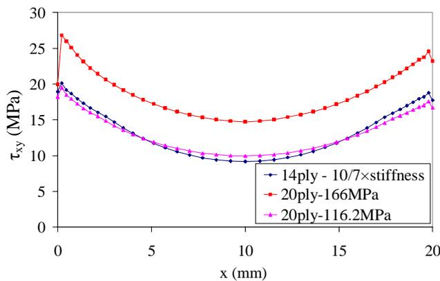
Fig. 7: Effect of thickness on shear stress
