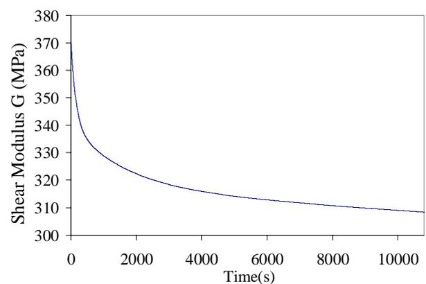
Fig. 2: FM1515 time dependent shear modulus.
