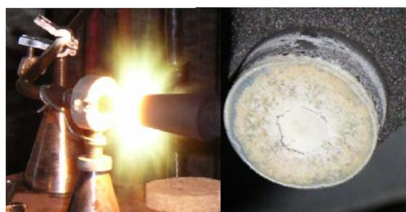
Fig.7 Photo of ablative facility and material surface after ablation
