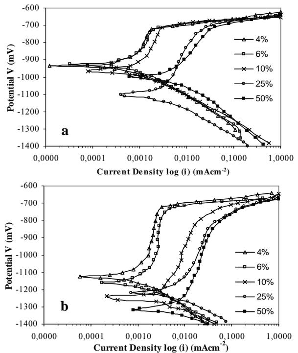
Fig. 3. Potentiodynamic polarization curves of 20% SiC composite according to cold-worked ratios in deaerated 3.5% NaCl solution
