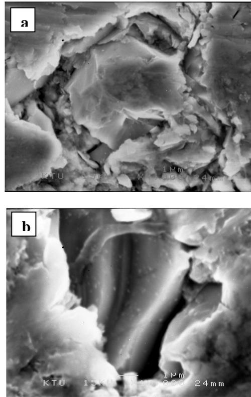
Fig. 8. a) Holes around of SiC particle due to intensive matrix corrosion, b) and free faceted of SiC particle in T8 tempered 20% vol. SiCp composite after corrosion
