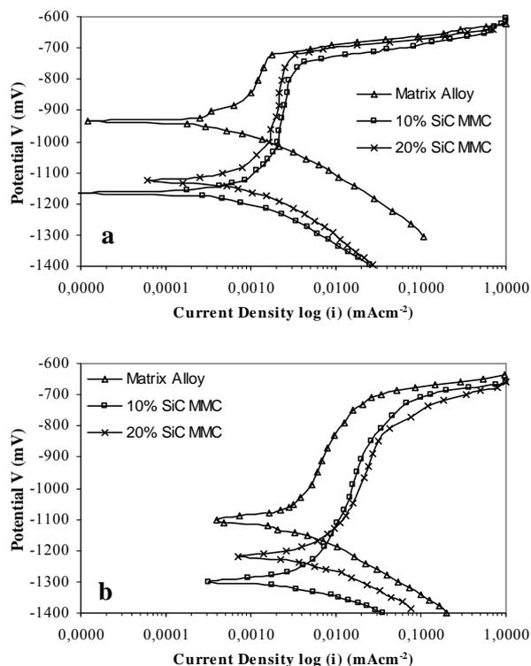
Fig. 4. Potentiodynamic polarization curves of cold-worked materials deaerated in a 3.5% NaCl solution a) 4% and b) 25%
