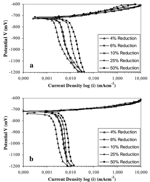
Fig.1. Potentiodynamic polarization curves of a) matrix alloy and b) 20% SiC composite according to cold-worked ratios in aerated 3.5% NaCl solution
