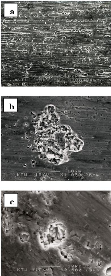
Fig. 6. SEM images of the 25% cold-worked a) matrix alloy and b) 10%, c) 20% vol. SiC composites after corrosion tests
