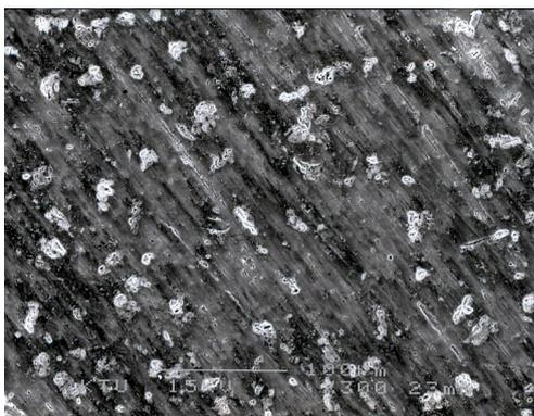
Fig. 7. Preferentially corrosion formed around SiC particles in 4% cold-worked 20% vol. SiCp composite
