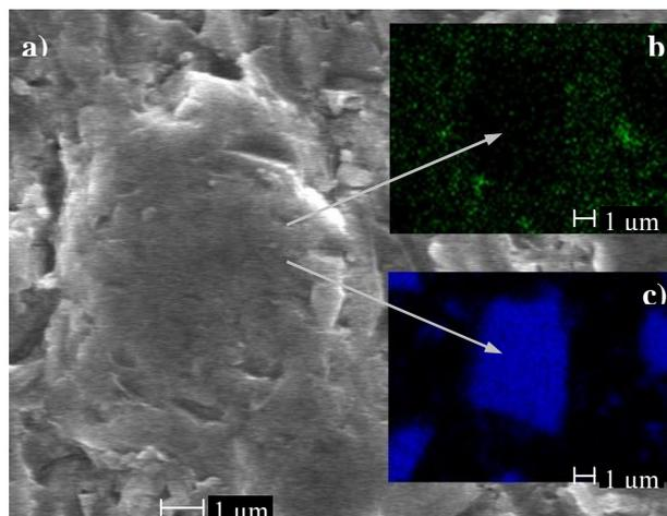
Fig. 5. a) SEM micrograph and X-ray maps of b) Mg, c) Si after T8 temper of the 20% vol. composite
