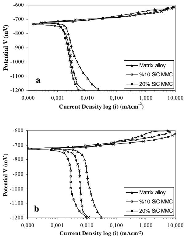
Fig. 2. Potentiodynamic polarization curves of cold-worked materials aerated in a 3.5% NaCl solution a) 4% and b) 25%
