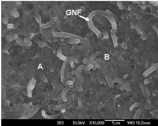
Fig. 4. SEM image observed on GNF cluster in hybrid MMC.
