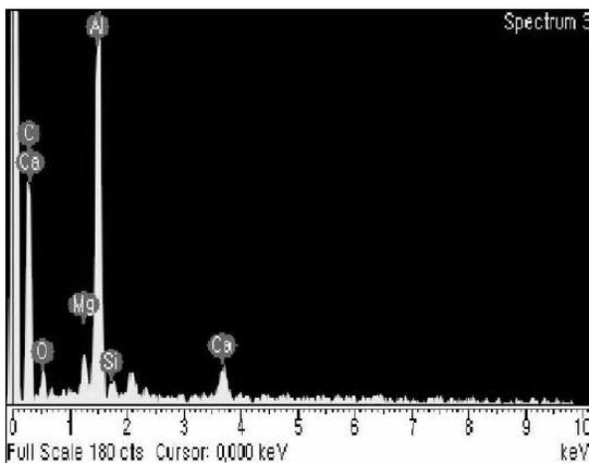
Fig. 5. EDX analysis of hybrid MMC, Position A in Fig 4.
