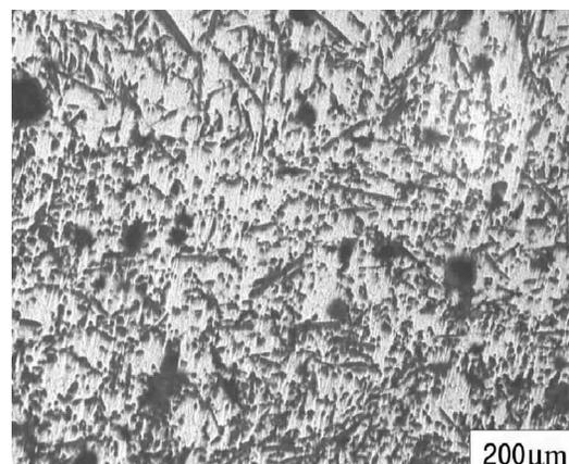
Fig. 2. Optical micrograph of GNF- $\text{Al}_2\text{O}_3$ /A356 hybrid composite.
