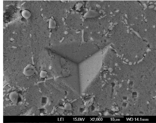
Fig.6. SEM image of nanoindentation observed on hybrid MMC.
