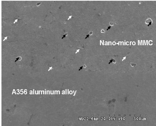
Fig. 3. SEM image of nano-micro MMCs. GNF/ $Al_2O_3$  dispersion in A356 aluminum alloy, GNF (black arrows),  $Al_2O_3$  (white arrows).
