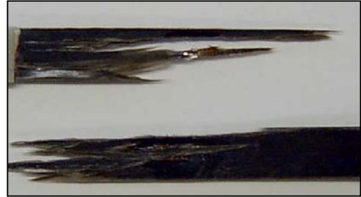
Fig. 6. Fractural behaviour of unidirectional composite
