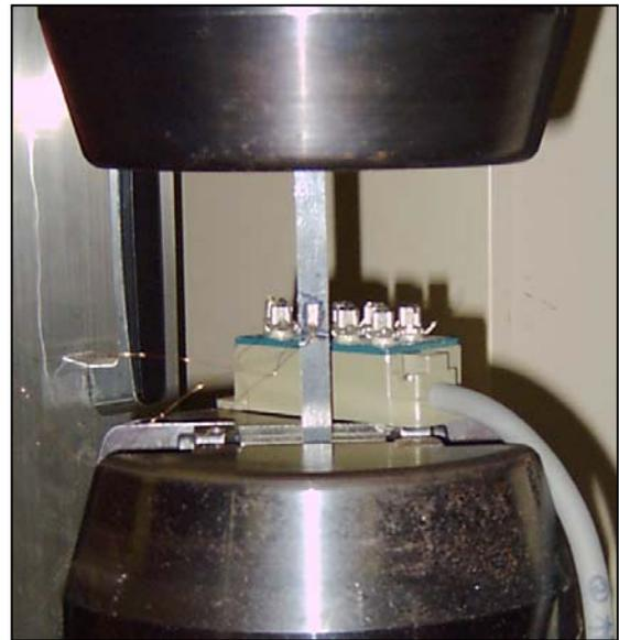
Fig. 5. Tension test setting
