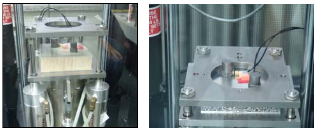
Fig. 2. The fixture of GA type jig and glass/epoxy and balsa core
