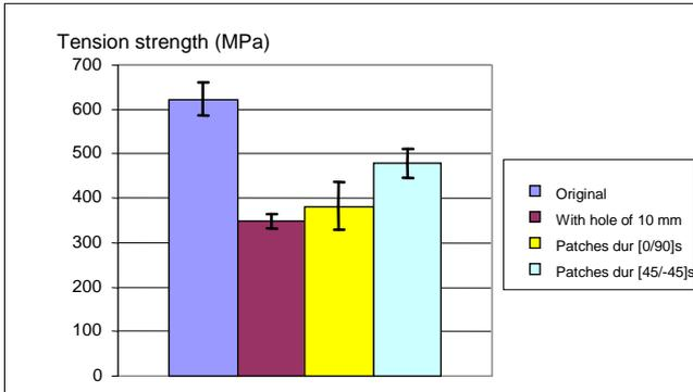
Fig.5. Tension strength of specimens repaired by « hard » patches
