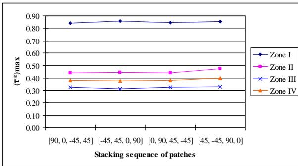
Fig. 17  $(\tau^*)_{\max}$  vs. fibre angle for patches in series II
