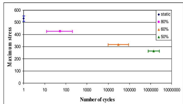
Fig. 8. S-N Results for patched specimens
