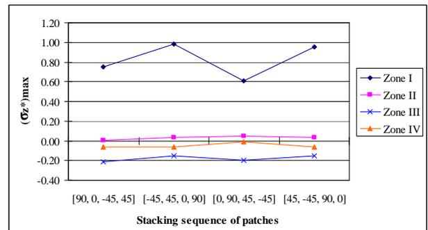
Fig.15  $(\sigma_z^*)_{max}$  vs. fibre angle for patches in series II
