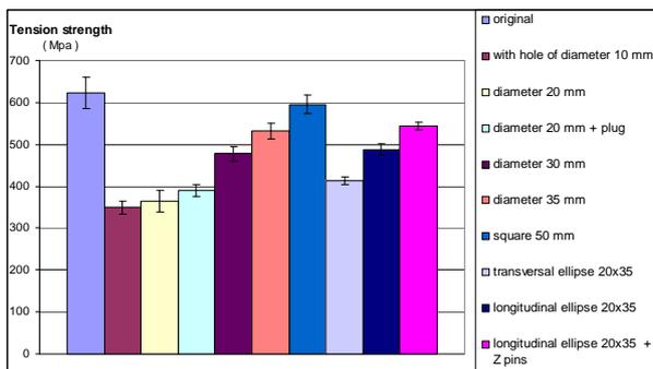
Fig.3. Tension strength of specimens repaired by « soft » patches
