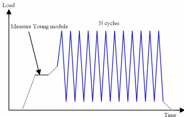
Fig. 6. Fatigue test loading
