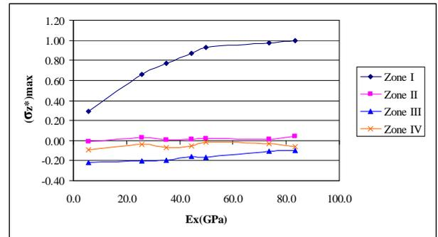
Fig. 14.  $(\sigma_z^*)_{max}$  vs.  $E_x$  for patches in series I
