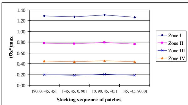
Fig.13  $(\sigma_x^*)_{max}$  vs. fibre angle for patches in series II
