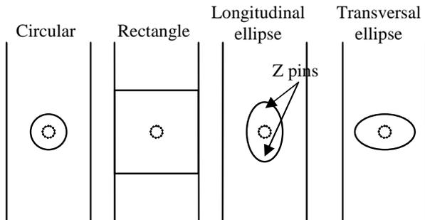
Fig. 2. Geometry of bonded patches
