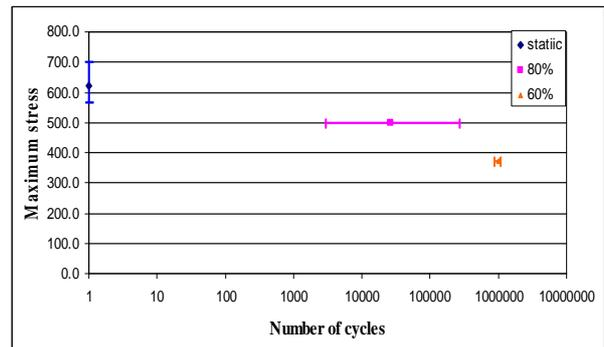
Fig. 7. S-N Results for undamaged specimens
