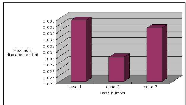
Fig. 5. Maximum displacement of structure Case 1: homogeneous fiber volume fraction and isotropic fiber orientation Case 2: left-located precharge condition Case 3: right-located precharge condition
