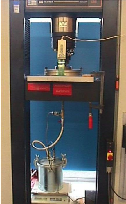
Fig. 1. Experimental facility, aluminium platens mounted in Instron frame with TekScan sensor.
