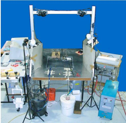
Fig. 6. Experimental Resin Infusion facility.
