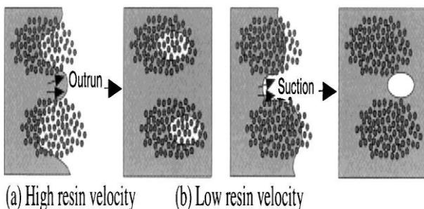
Fig. 1 Scheme of air bubble formation
