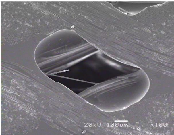
(b) SEM photograph (3D fabric of glass fiber/Phenolics)
