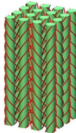
Fig. 2. A hypothetical hybrid 3-D braid with braided carbon nanotube yarns
