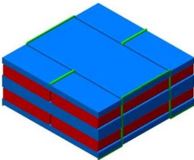
Fig. 1. A hypothetical hybrid 3-D orthogonal weave with Z-directional carbon nanotube yarn [1]
