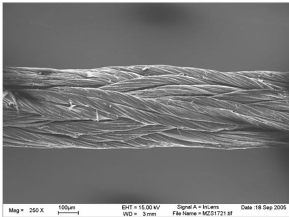
Fig. 4. SEM of 3-D braid made from 36 five-ply nanotube yarns [4]
