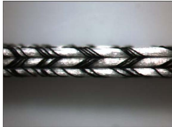
Fig. 5. Hybrid glass fiber/carbon nanotube yarn 3-D braid, 40x magnification
