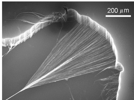
Fig. 3. SEM image of a carbon nanotube yarn being drawn with twist from a carbon nanotube forest [2]
