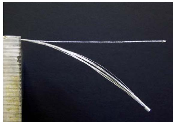
Fig. 6. Illustration of comparative bending stiffness of the hybrid 3-D braid and the bundle of individual S-2 glass fibers
