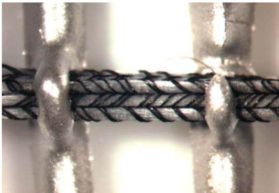
Fig. 7. Test setup for a dry hybrid 3-D braided material with electrical contacts
