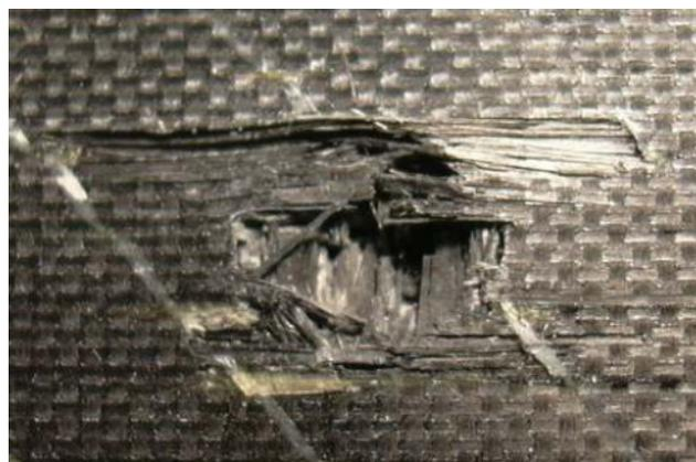
Fig. 4. Front face of a CF XP 4.16mm thick coupon impacted at normal incidence and at a speed of 293m/s.
