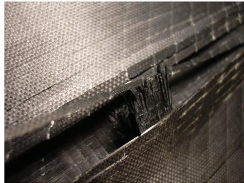
Fig. 6. Detail of the back face of a CF XP 4mm sample impacted at 295 m/s (ballistic limit) at 40° incidence.
