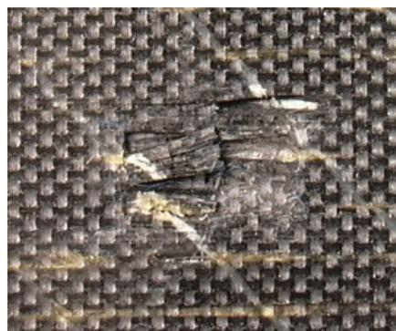
Fig. 3. Detail of the impact point in a CF QI 2.15mm coupon impacted at 161m/s.
