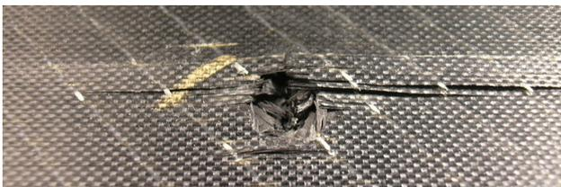
Fig. 5. Detail of the front face of a CF QI 4.16mm thick coupon impacted at 317 m/s with 40° incidence.
