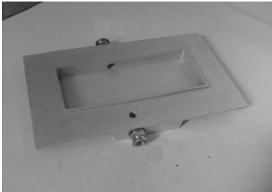
Fig. 2. Mould for the permeability measurements
