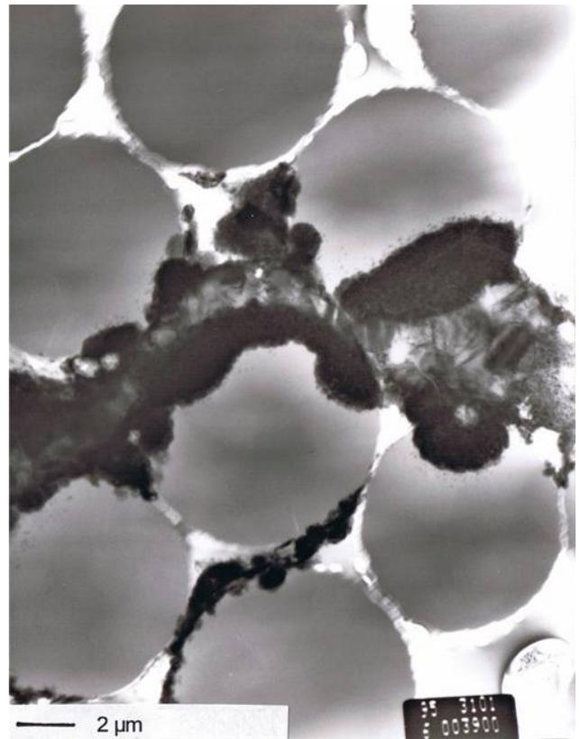
Fig. 10c; C/C-SiC; TEM micrograph of a Si-infiltrated crack area
