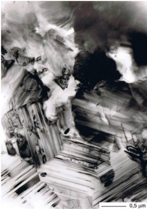
Fig. 10d;  $\beta/\alpha$ -composite crystals in a central crack area
