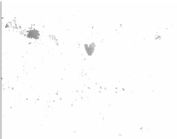
Fig. 1(b). Image after intensity adjusting, leaving black area as voids while resin and fibres are white
