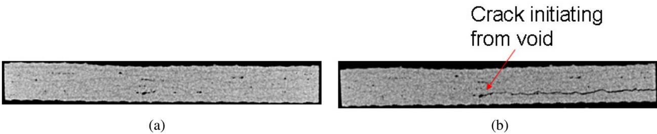
Fig. 7. X-ray tomography images of cross-sectional view for specimen 6.2 (a) before and (b) after loading
