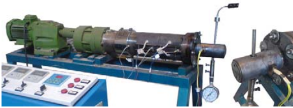
Figure 7 View of executive setup for capillary dilatometer
