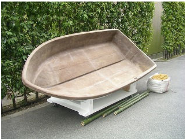
Fig.2 Photograph of a BFRP pleasure boat
